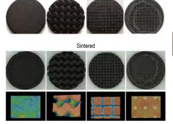
FIGURE 2. Photographs showing four of the printed electrode geometries currently being tested before and after the sintering and debinding process. The electrodes pictured are to be the battery anodes and are printed using a custom hard carbon resin.
