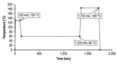
FIGURE 1. Temperature profile for curing rectangular sheet for tensile test coupons.
