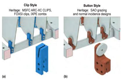
FIGURE 1. (a) Clip-style and (b) button-style mounts for nested mirror shells.
