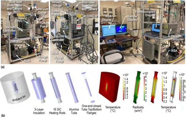
FIGURE 1. (a) Three different views of the THVC's test stand designed and built in-house at MSFC. (b) Material domains and results of the comprehensive 3D THVC's model built to determine the optimal location of the one-closed-end tube housing the sample to obtain the largest temperature gradient along the tube's wall to boost thermal Marangoni effect.
