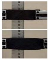
FIGURE 2. Expansion of auxetic foam material in transverse direction, after being stretched.
