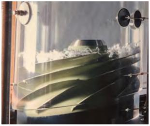
FIGURE 1. Cavitating inducer.
