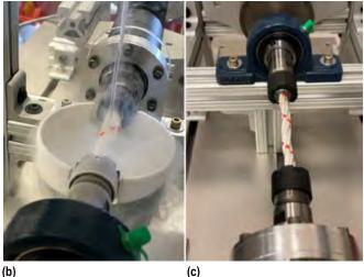
**FIGURE 2.** A 3-in-long, 11-mm-diameter liquid crystal polymer braid (a) doubled its torsional stiffness when (b) exposed to  $LN_2$  temperatures as compared to (c) ambient temperatures.
