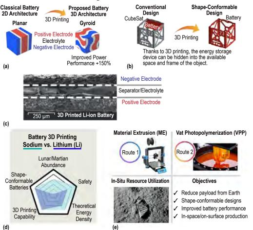
**FIGURE 1.** 3D printed architectures allow for complex electrode geometries and shape-conformable deigns as this team has previously demonstrated with printed lithium-ion batteries. This project pursues two printing routes, ME and VPP, with a focus on sodium-ion chemistries due to their improved safety and higher availability in-situ on the Moon and Mars.
