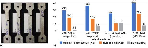
FIGURE 1. (a) AW-DED AI 2319 0° test specimens; (a) Comparison of AM 2319 test data to wrought 2219.
