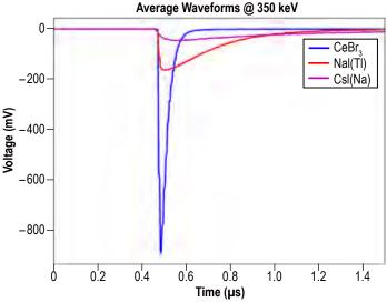
FIGURE 1. Pulse amplitude versus time for 350 keV photon signals in three scintillator materials.
