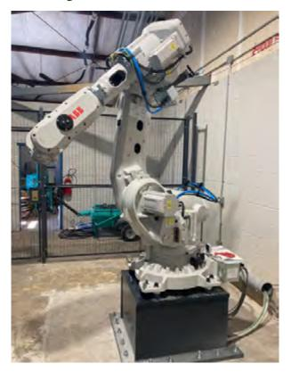
FIGURE 1. Assembled research printer robotic arm.
