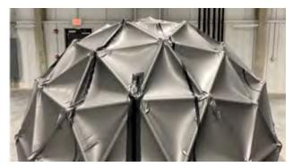
**FIGURE 3.** Prototype EE low pressure testing at  $\Delta P$  of 0.3 atm.
