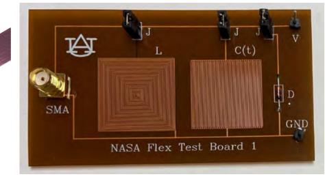
FIGURE 1. Printed passive wireless sensors for remote sensing applications.
