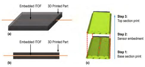
FIGURE 1. Schematic representation of the (a) embedded ITOF in a 3D-printed ABS composite, (b) cross-sectional view, and (c) manufacturing process.
