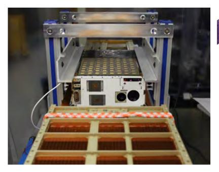
FIGURE 2. The NEA Scout was successfully loaded into the flight dispenser, which will deploy it once the Orion Stage Adapter has separated and is on its way to the Moon.
