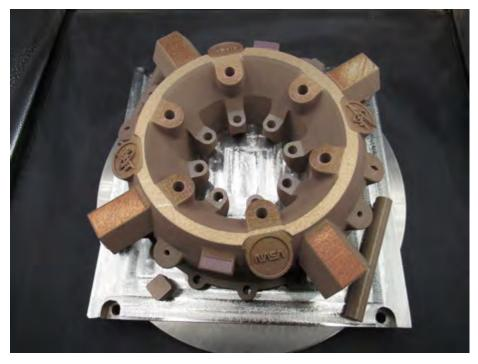
**FIGURE 2.** NASA RDRE powder bed fusion GRCop-42 injector.
