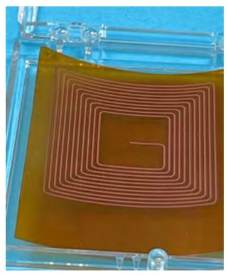
FIGURE 2. Printed copper antenna pattern on flexible substrate.
