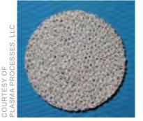
FIGURE 1. Monolithic Iridium foam disk.
