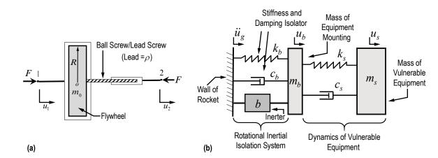
FIGURE 1. (a) Example diagram of an inerter and (b) example configuration of an isolated system with a rotational inertial device.
