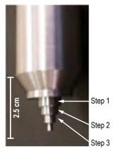
**FIGURE 2.** Close-up of the FSW tool showing the shoulder (step 1) and backing anvil (step 3).
