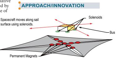
FIGURE 1. Conceptual overview of electromagnetically coupled solar sail.
