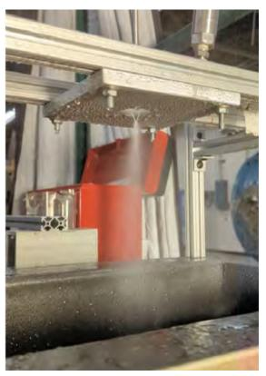
**FIGURE 2**. Spray testing of fluidic diode integrated injector element.
