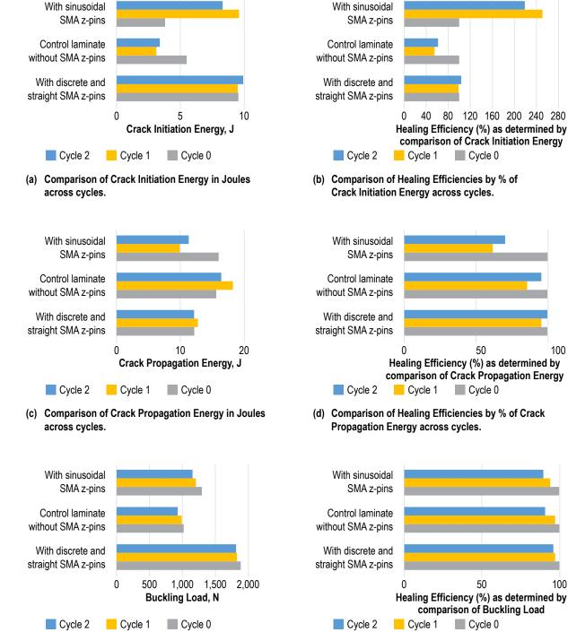
(e) Comparison of Buckling Load in Newtons
