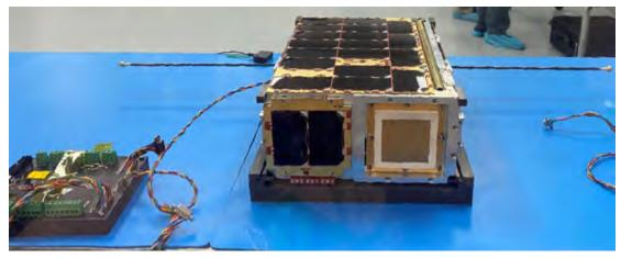
FIGURE 2. Final functional test of the SPORT CubeSat.
