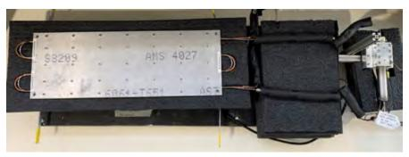
FIGURE 2. Benchtop testing of additively manufactured loop heat pipe.
