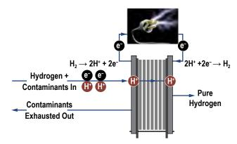
FIGURE 1. Electrochemical hydrogen separator.
