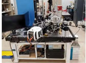
FIGURE 1. Portable electrostatic levitator.
