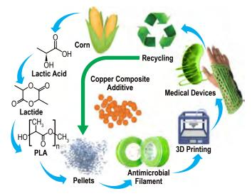
**FIGURE 2.** Manufacturing process of antimicrobial medical devices using a biodegradable antimicrobial 3D printing filament.
