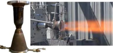
FIGURE 1. 2k-lbf coupled bimetallic AM chamber with composite overwrap completed testing in 90 days.
