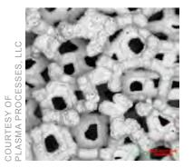
FIGURE 2. Scanning electron microscopy image of Iridium foam showing the unit cell.
