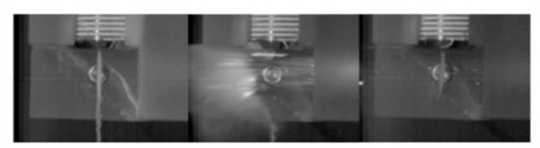
FIGURE 1. Experimental demonstration of passing detonation wave with liquid jet.
