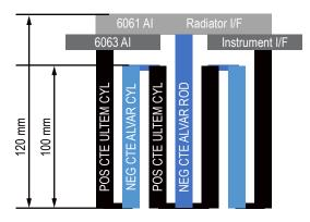
FIGURE 1. Cross sectional diagram of the TSW showing positive and negative CTE materials.
