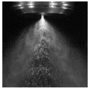
FIGURE 1. Spray testing of high-performance additively manufactured injector element.
