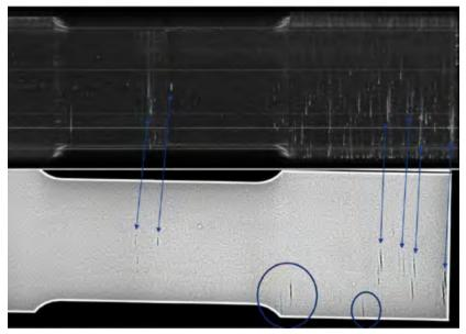
FIGURE 2. Comparison of thermal in-situ monitoring indications with an x-ray image of the part.
