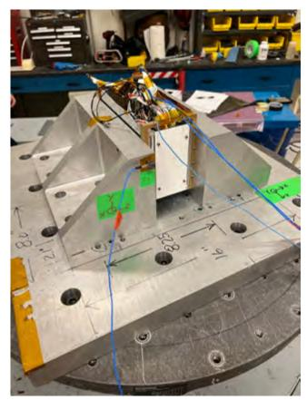
FIGURE 1. LISA-T flight payload under vibrational test.
