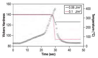
**FIGURE 1.** KWN predicted evolution of the hardness of AA2219-T87 during a simulated SR-FSW thermal cycle interrupted at 400 °C, with varying interfacial energy.
