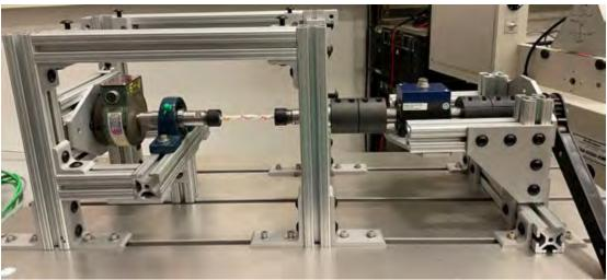
FIGURE 1. The CiBEHR static test rig is capable of testing prototype braided couplings to 50 N·m and 500 lbf.
