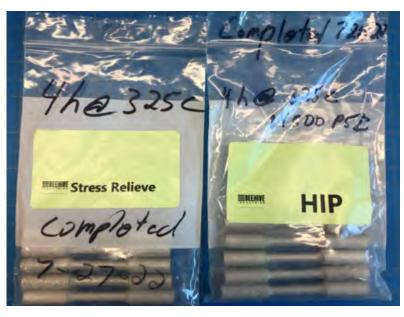
FIGURE 1. L-PBF AM Scalmalloy mechanical test specimens after heat treatment.
