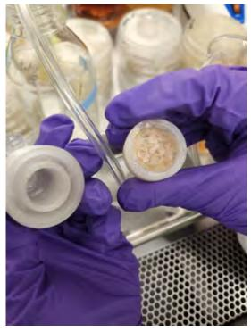
**FIGURE 1.** As part of a flight project analysis, biofilm re-capturing hardware from the wastewater stream is being studied.
