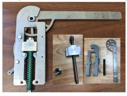
FIGURE 1. Sear release mechanism parts ready for assembly.
