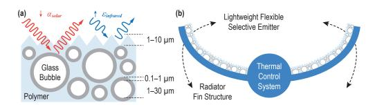
**FIGURE 1.** Proposed material and concept system designs. (a) The combination of glass bubbles and surface texture allows selective optical control that minimizes solar absorption and maximizes infrared emission; (b) The lightweight flexible selective emitter could be integrated with radiator fin or inflatable habitat structures and enable breakthroughs in thermal control of deployable and flexible systems.
