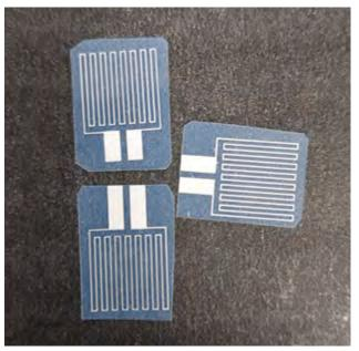
FIGURE 1. Printed strain sensor for monitoring of vehicle Structural Health.
