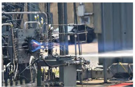
**FIGURE 1.** NASA additively manufactured GRCop-42 RDRE firing with liquid oxygen (LOX)/methane (CH<sub>4</sub>).
