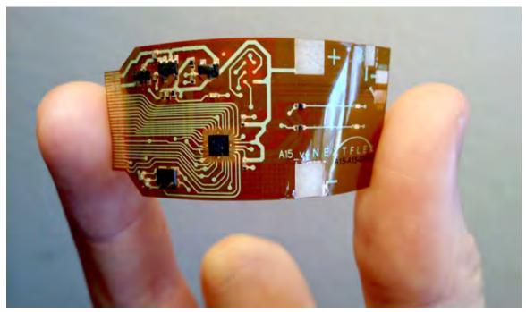
FIGURE 1. Flexible wireless printed circuitry for sensor networks.
