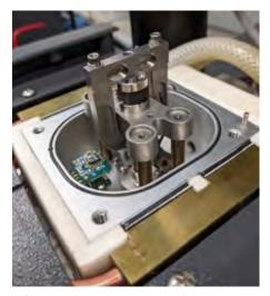
FIGURE 3. A square sample of auxetic foam mounted between two circular platens (each 15 mm diameter) in the DMA 2980 compression clamp.
