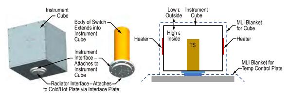
FIGURE 2. Diagrams of test set up for all thermal cycle tests.
