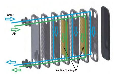
FIGURE 1. Schematic showing the wetted pathways of the RC-TSA bed design.
