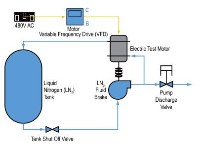
FIGURE 1. This simplified AIDEM schematic shows it only requires control input to motor speed and discharge valve position to characterize high-speed electric motors.
