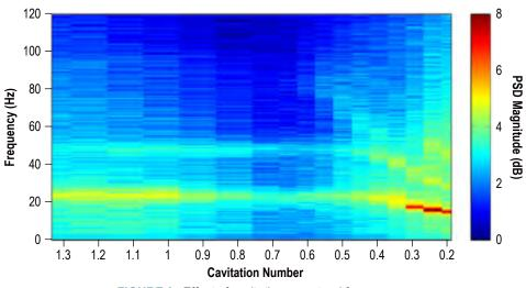
FIGURE 3. Effect of cavitation on natural frequency.
