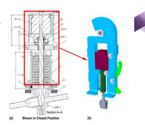
release or would only partly release. It also proved to be difficult to prepare to test and to reset after testing. As the use of rapid actuated pyro-type valves are being considered for groundbased water hammer and surge testing, ER14 proposed a redesign of the AMed isolation valve using a more robust sear release system to improve on the valve's operational performance.
