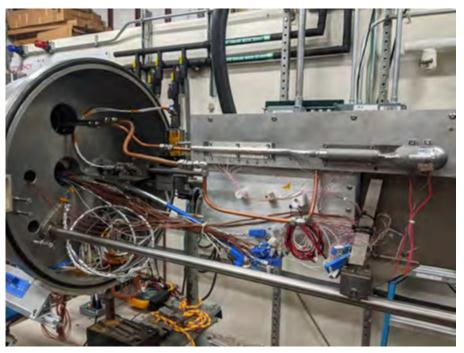
FIGURE 1. Warm-reservoir variable conductance heat pipe in thermal vacuum chamber.
