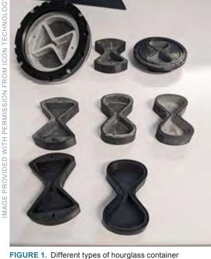
The Duneflow hardware consists of avionics, lighting, cameras, and six vacuum-capable cells with hourglass-shaped containers that are rotated with motors at a specific spin rate during the two minutes of lunar gravity of the suborbital flight. Cameras and lighting will allow visualization of the flowability and angle of repose of the simulant materials and regolith. The Duneflow flight is currently scheduled to occur in January 2023.
