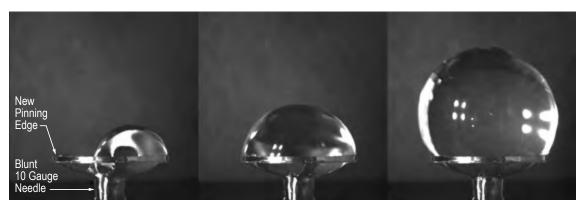
**FIGURE 2.** A series of images demonstrating the ability of a new delivery tube design to dispense a liquid bubble while maintaining integrity of the pinning edge. As shown from left to right, the asymmetric process of a moving liquid front stabilizes or pins at the edge of the delivery tube and proceeds to grow symmetrically as a large bubble.
