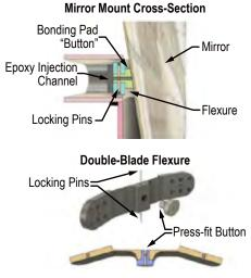
FIGURE 2. Single-shell mirror mounting design diagrams showcasing double-blade flexure.
