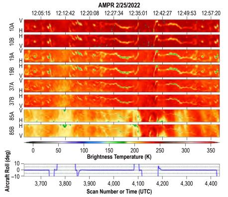
**FIGURE 1.** Strip chart showing one hour of data from an AMPR flight on 25 February 2022. Shown are brightness temperatures from each of AMPR's 8 channels, as well as a time series of aircraft roll angles. When roll angle is near 0° AMPR data are useful for scientific analysis.
