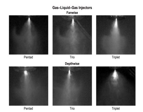
FIGURE 2. Spray pattern comparison of different additively manufactured injector element schemes.
