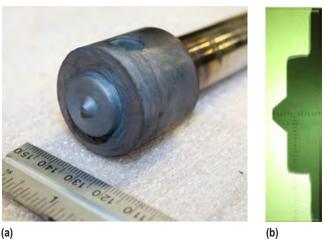
**FIGURE 1**. (a) FSW tool after 35 cm of weldment and (b) overlay showing no appreciable change from original tool geometry.
