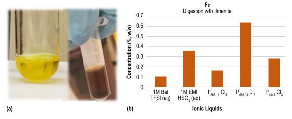
**FIGURE 1.** (a) Image of ionic trihexyl(tetradecyl)phosphonium pentachloride ( $P_{666,14}Cl_5$ ) before (left) and after (right) ilmenite digestion. (b) Comparison of iron (Fe) extraction from ilmenite with selected ionic liquids.
