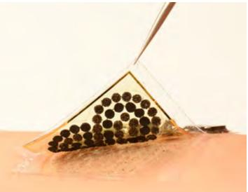
FIGURE 1. Printed biofuel cell for harvesting energy from human sweat.
