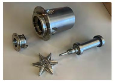
**FIGURE 2.** Hardware manufactured for a 30,000 rpm AIDEM water brake prototype.
